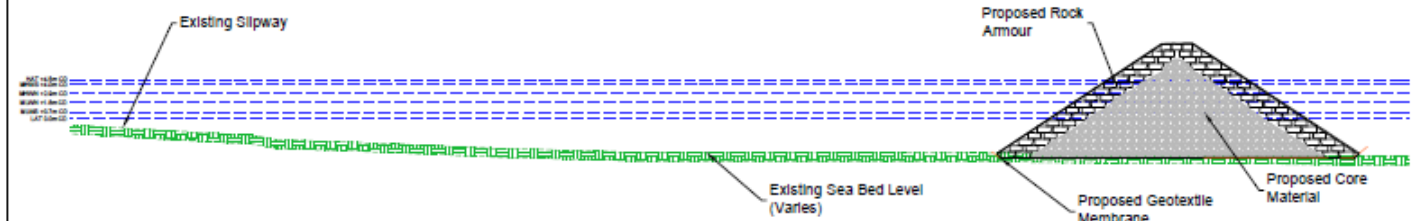
Cross-Section Through Proposed Breakwater (Scale 1:500)
